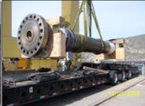
Hydropower water turbine, Dimensions: 30' x 6' x 6' 145,500 pounds
